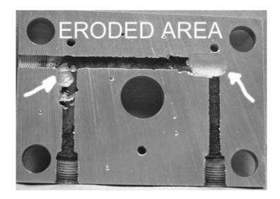
Figure 8. Photo of an aluminum SCR cooling block showing Erosion
