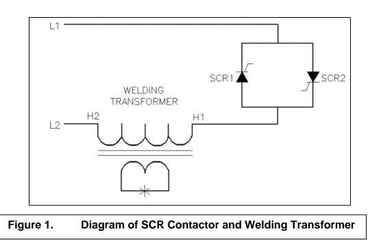
When connected in this way and used in resistance welding controllers, SCR's are typically called a Contactor or A.C. Switch. [1]
