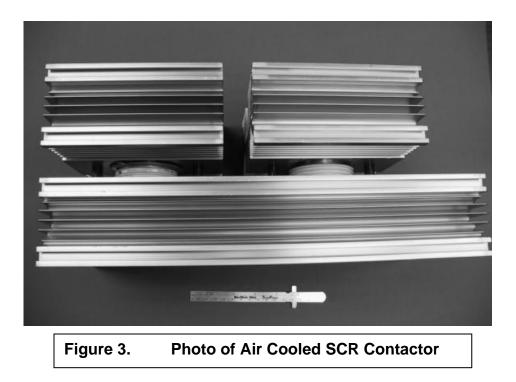
These extrusions typically have many fins, to increase surface area. The more the surface area the higher the heat dissipation or the lower the thermal resistance from the heat sink surfaces to ambient air. Adding fans or blowers increases the efficiency as well.
